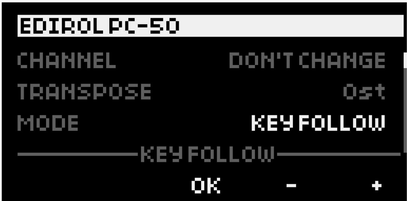
The **KEY FOLLOW** mode transforms MIDI notes into **Control Change (CC)** messages, allowing dynamic control of parameters based on played notes. This mode is ideal for creating expressive modulations or mapping specific note ranges to control values. If the **MUTE NOTE** parameter is disabled, the original MIDI notes will also pass through MONOLIT alongside the generated CC messages.
