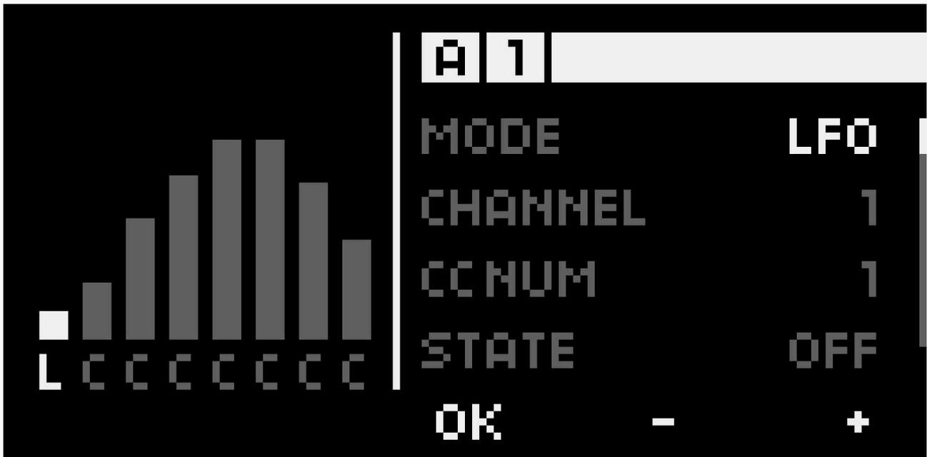
The LFO mode enables the usage of a slider as a low-frequency oscillator to modulate controlled parameters.
