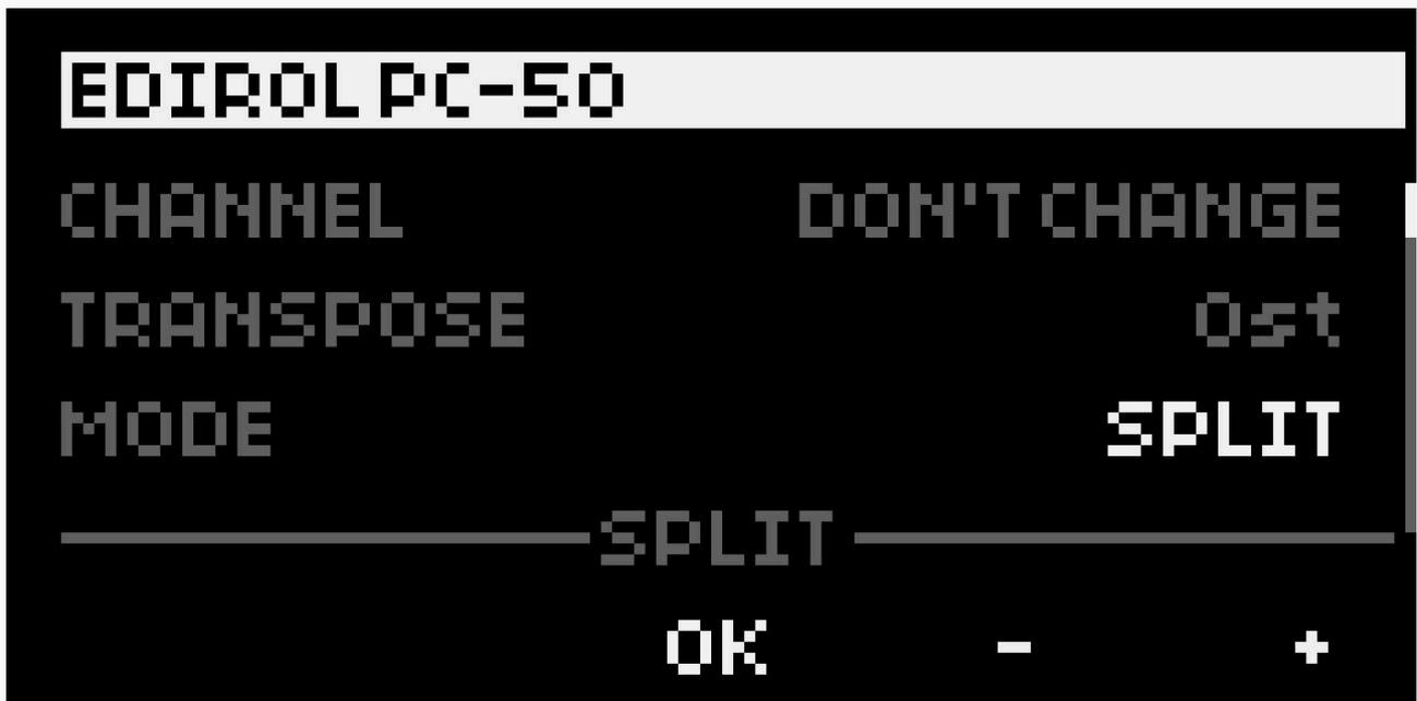
**SPLIT** mode divides incoming MIDI notes into two layers: lower and upper. Each layer is assigned a specific range of MIDI notes, which can be routed to different MIDI channels. This allows you to play and control two separate instruments or sounds simultaneously using a single MIDI keyboard. For example, the lower layer could control a bass sound on one synth, while the upper layer plays a lead sound on another synth.
