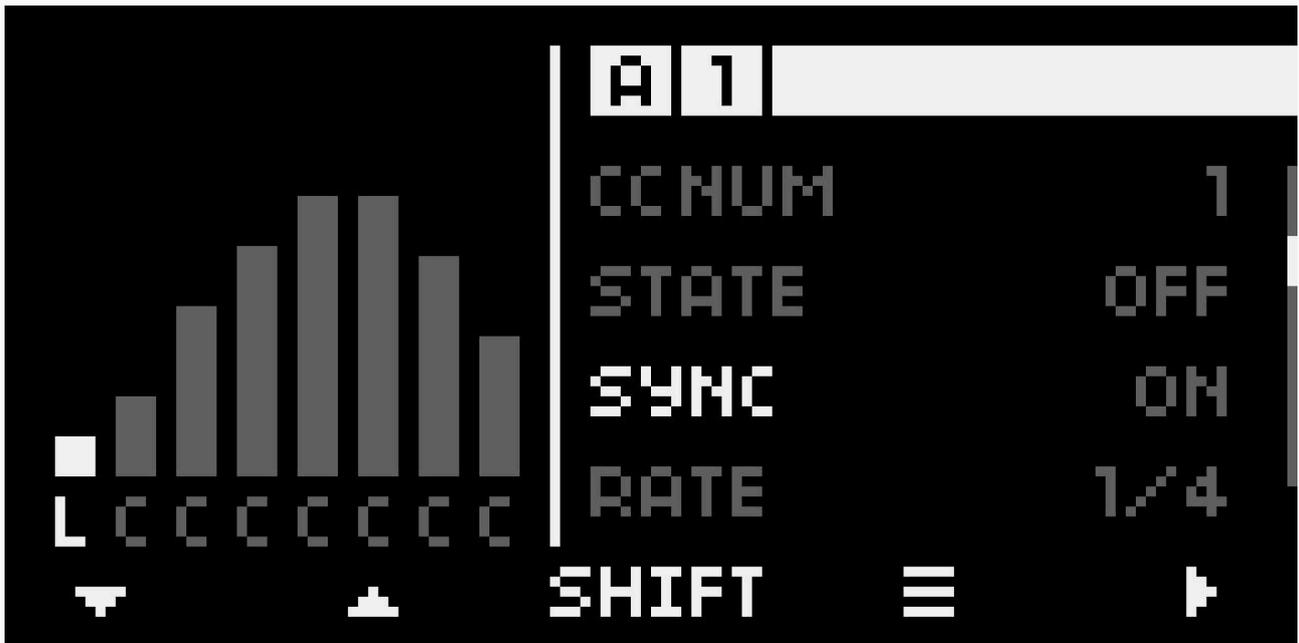
The **LFO SYNC** function allows you to synchronize the Low-Frequency Oscillator (LFO) speed with MONOLIT's internal clock or an external MIDI clock. To activate the internal clock, press **SHIFT + START** on the main screen, and to stop it, press **SHIFT + STOP**.
