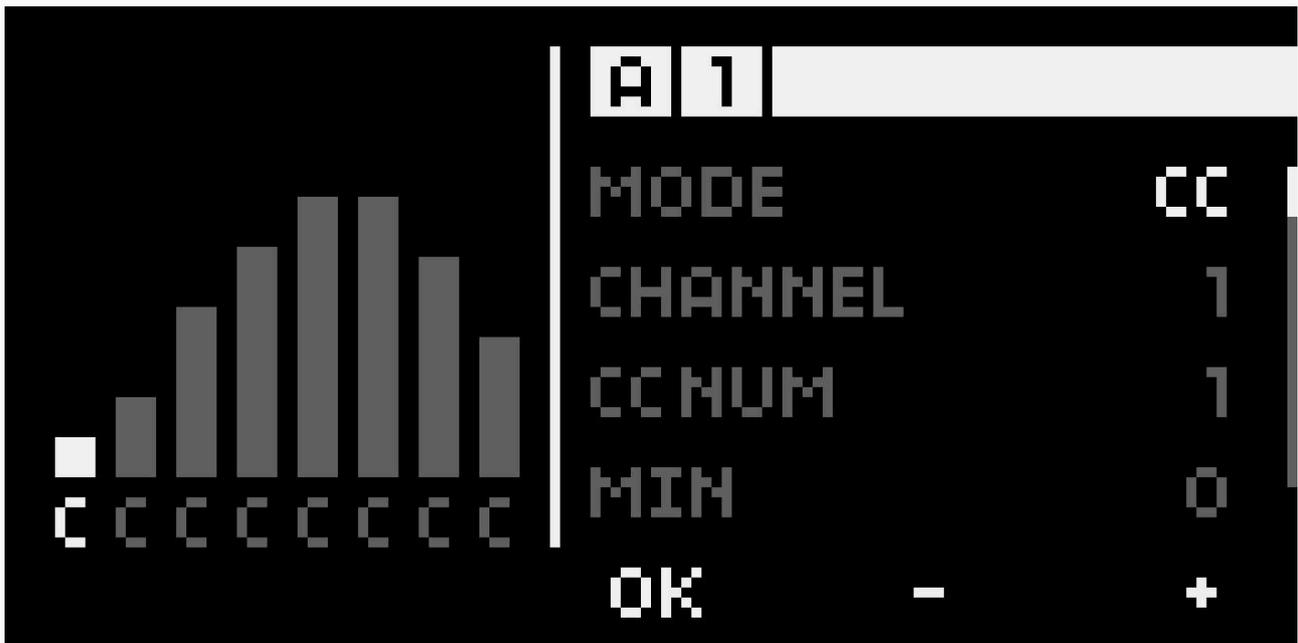
Control Change mode allows changing the parameters of controlled devices.
