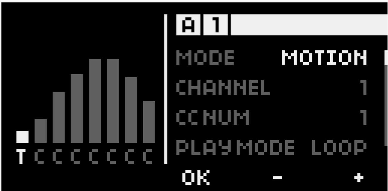
Motion mode allows you to record the motion of a slider and play it back to create expressive automation of the modulated parameters. Motion is recorded when the button is held, and the slider is moved.
