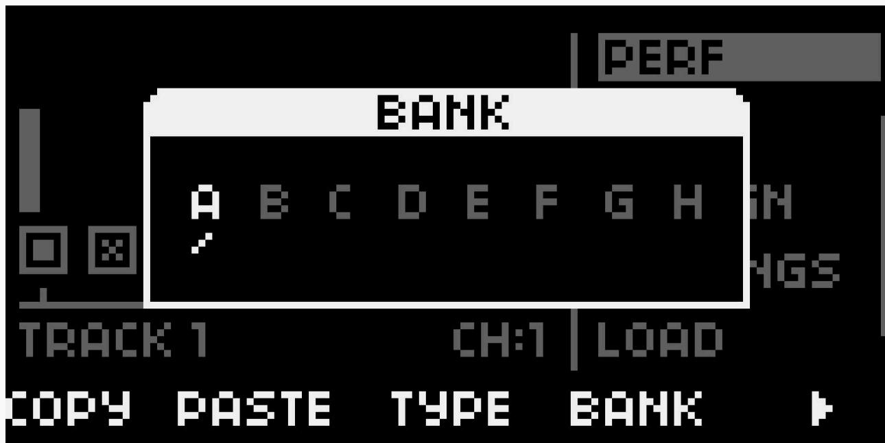
To change a bank type, simply press the **TYPE** button when selecting a bank.
