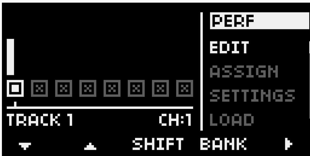
Starting from version 2, each bank can operate either in Slider mode or Performance Mode.
