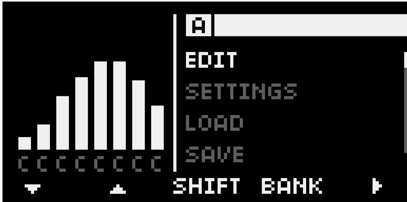
On start up, **MONOLIT** assigns all eight sliders and eight buttons to **CC mode** (Control Change mode). In this mode, you can adjust parameters on your connected MIDI devices.
