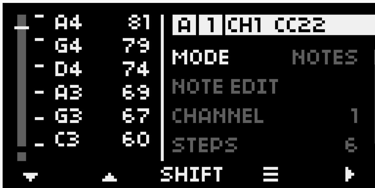
The NOTES mode enables a slider to send MIDI notes once a specific section or point on the slider is reached.
