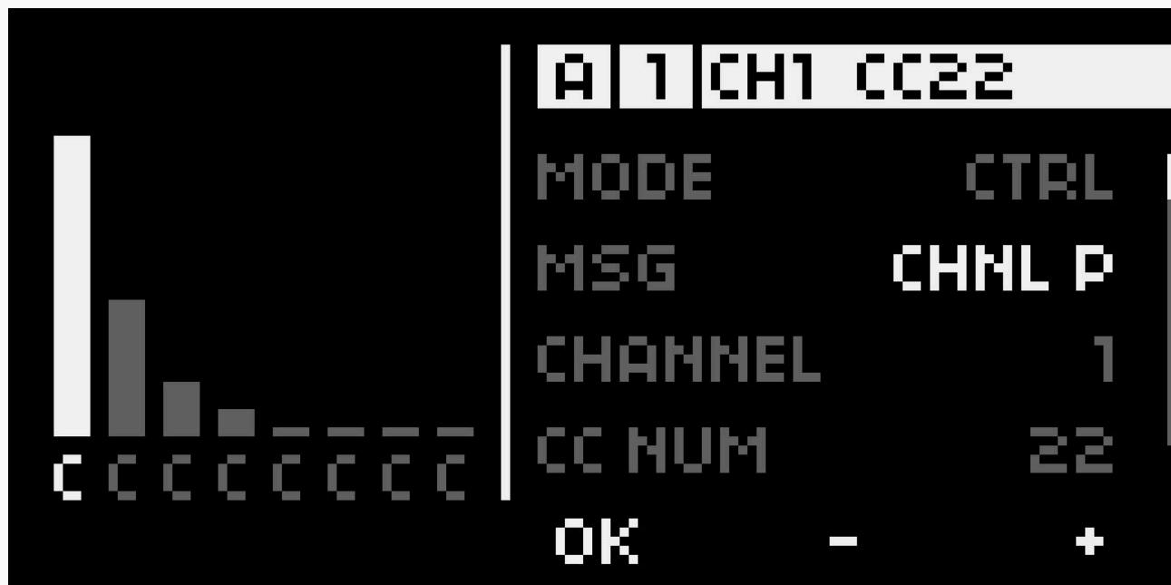
CTRL mode lets you assign a specific MIDI message type to a control for direct and flexible parameter manipulation.
